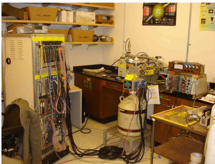
Fig. I-51. The polarization experiment installed and running at LBNL. The rack of GRETINA digital electronics is on the left of the picture.
